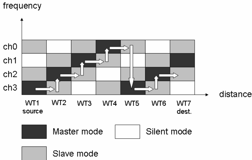
Figure 4.1: The channels and modes in the KMH mechanism.
