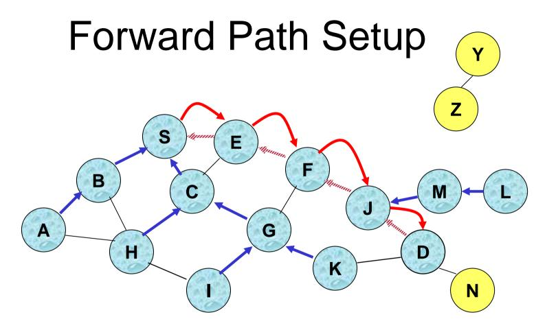
Forward links are setup when RREP travels along the reverse path
