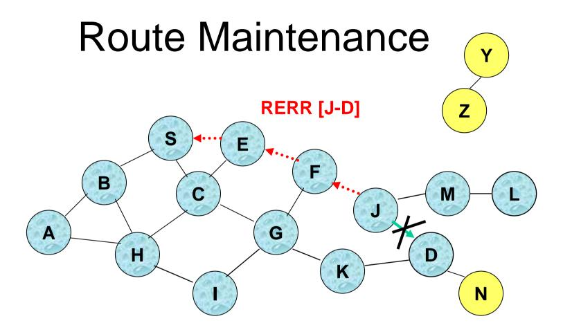
J sends a Route Error (RERR) to S along route J-F-E-S when its attempt to forward the data packet S (with route SEFJD) on J-D fails
