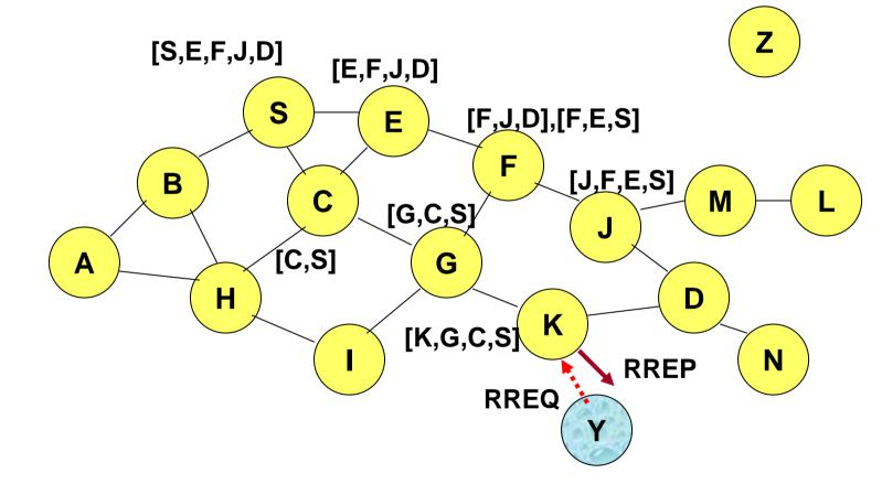
Assume that there is no link between D and Y. Route Reply (RREP) from node K limits flooding of RREQ.
