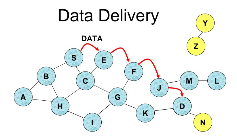
Forward route entry in routing tables are used to forward data packet. Route is *not* included in packet header.
