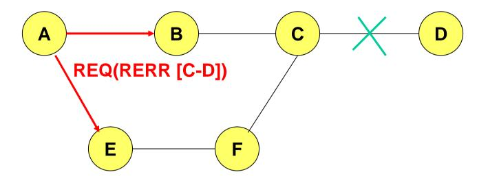
A piggybacks a copy of RERR to the REQ, ensuring that any RREP in response does not contain a route that assumes the existence of link C-D.
